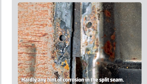
Hardly any hint of corrosion in the split seam.
