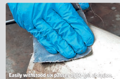
Easily withstood six passes of 80-grit abrasion.
