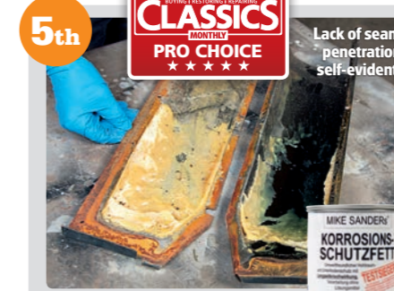
The most corrosion witnessed on test.
