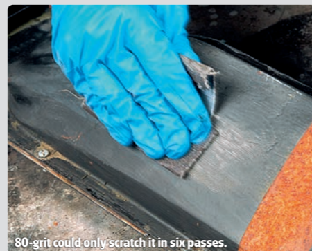
80-grit could only scratch it in six passes.
