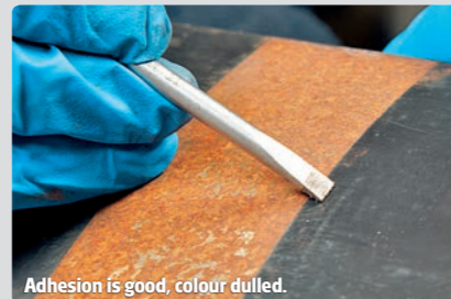
Adhesion is good, colour dulled.
