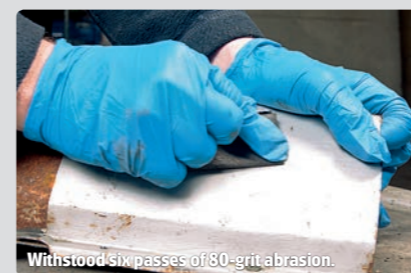
Withstood six passes of 80-grit abrasion.
