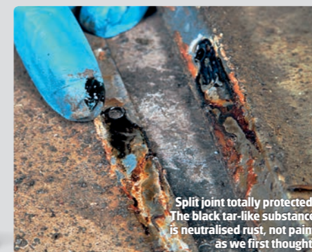
Below the surface, the steel remains well protected.
