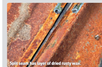
Split seam has layer of dried rusty wax.
