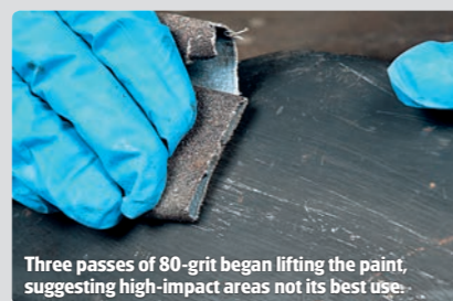
Adhesion is good, colour dulled.
