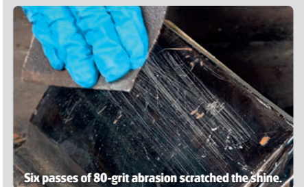
Six passes of 80-grit abrasion scratched the shine.
