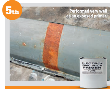
Adhesion intact but surface not very strong.
