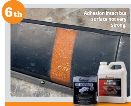
The only tested product to peel off.
