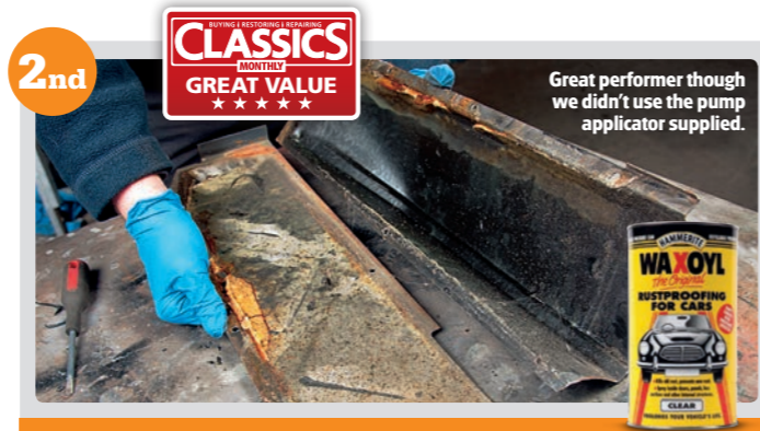
Excellent exposed surface protection. Seams showing signs of light surface corrosion starting.
