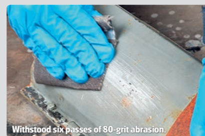
Withstood six passes of 80-grit abrasion.
