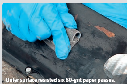
Outer surface resisted six 80-grit paper passes.
